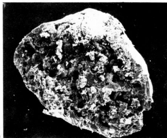
Figure 4: An acetaminophen granule produced by a rotary fluid-bed processor, at a magnification of 60X. Figure 4a shows the surface of the granule; Figure 4b shows the cross-section, which reveals the interstitial void space.
